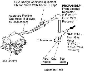
Figure 17 - Gas Connection (Remote-Ready Models Only)
